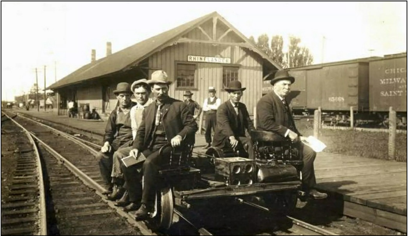
An early gasoline-powered hand car being used on the Minneapolis, St. Paul, & Sault Ste. Marie line for an inspection tour in 1908 in Rhinelander. Wisconsin Historical Society photo.
